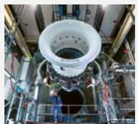
Put through its paces: a CF34 being rigged up for testing.
