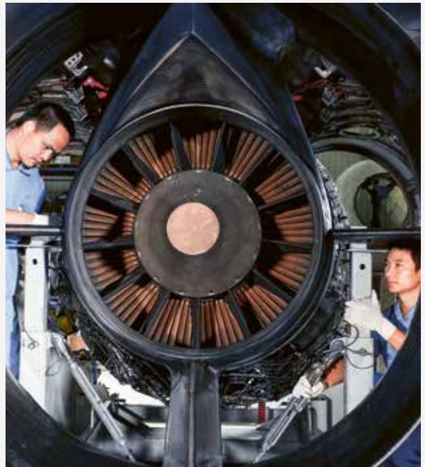
Everything under control: with a deft touch, a V2500 outlet nozzle is expertly assembled.
