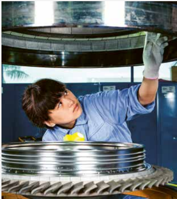
Precision has top priority at every step—here an MTU employee assembling a V2500 high-pressure turbine.
