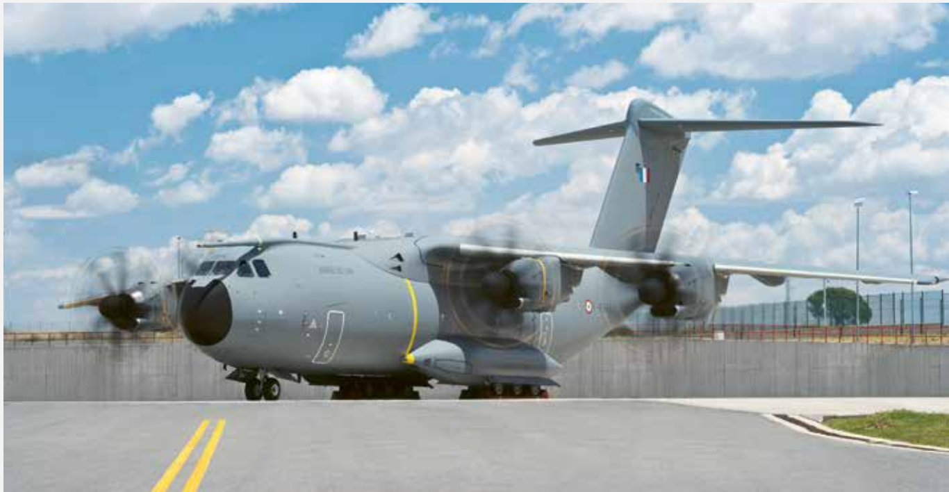
The A400M military transporter on the runway. With an output of 8,200 kW, its TP400-D6 engines are the most powerful turboprops in the Western world.
