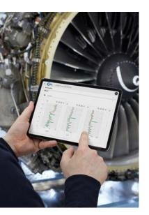
MTU's engine trend monitoring (ETM) is an independent and proprietary web application that monitors specific data sets from flight operations. We combine these with shop visit data. We introduced ETM in 2006 and continue to optimize the system – for instance, we recently introduced a web userface for all devices, new reporting functions and real-time visibility into the status of engines. The foundation is a full, MTU-developed thermodynamic engine model for each engine type.
